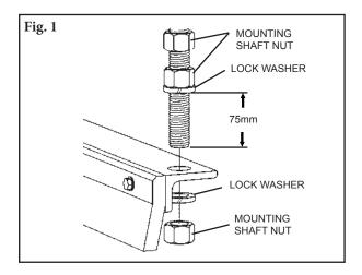
1. Loosen mounting shaft nuts. The bottom two mounting shafts nuts on both sides of the plough should be loosened so that the worn blade will have no tension to the belt (Fig 1.)
