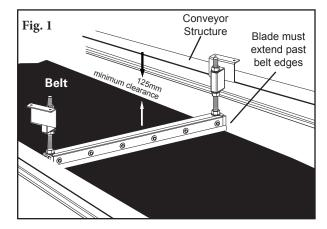
Position the plough frame on the conveyor. Slide the plough onto the belt in the selected location. Check for structure interference at both ends where the mounting brackets will be attached to the structure (Fig. 1).
