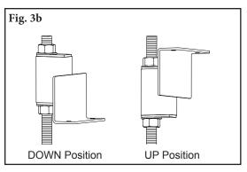
**4. Check performance.** Run the belt and check that the plough runs smoothly and has an effective cleaning action. A final adjustment may be required. To raise or lower the unit, adjust the nuts against the mounting bracket up or down.
