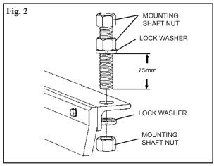
2. Attach the mounting shaft to the plough frame. Thread two mounting shaft nuts up the mounting shaft to expose between 50mm to 75mm of thread past the nut. Next place a lock washer against the lower nut and slide the mounting shaft down through the hole in the plough frame (Fig. 2). From the bottom side of the plough frame place a lock washer and mounting shaft nut on the mounting shaft and tighten. Repeat on opposite side.
