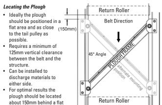
Physically lock out and tag the conveyor at the power source before you begin plough installation.
